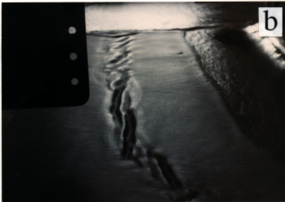
Figure 4. (a) Displacement transducer (topographic profiler) used to measure the topography of the wax surface. Variations in voltage from the transducer are digitized and recorded on a Macintosh computer. The device is linear over an 10 mm range and is precise to less than 10 \mu\text{m} . (b) The topographic profiler was used to measure the topography that develops at the free end of a cooling and thickening plate. Differential contraction of the cooling plate places the surface layer in compression and the second layer in tension. (This technique is also used to temper glass against surface cracks.) This continuous process creates a large thermal bending moment. At a free edge, the thermal bending moment causes the plate to flex downward.
