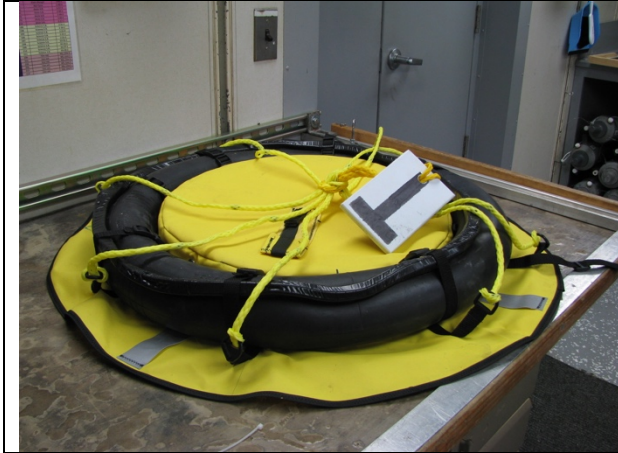
Figure 7. Photo of thermal blanket instrument. The instrument consists of a porous fabric covering a porous and pliable foam interior surrounded by a 17 inch diameter motorcycle inner tube filled with calcium chloride for weight with an additional lead weight ring. Two autonomous thermal sensors are mounted on each side of the blanket.
