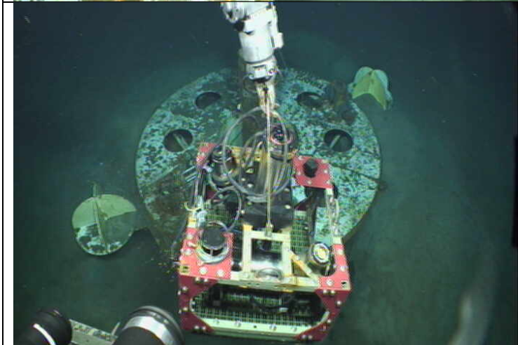
Figure 17. Recovery of the optical communication sled after unplugging from the CORK.
