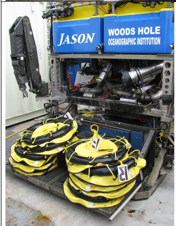
Figure 8. Thermal blankets loaded onto the front basket of Jason. It turns out that these need to be very securely down for launch and recovery.
