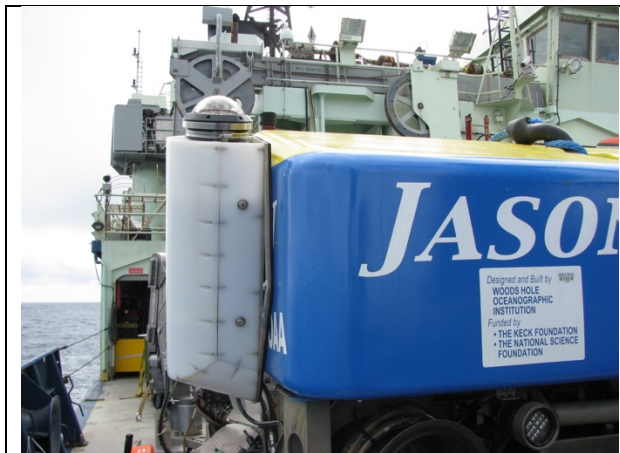
Figure 6. Photo of optical communication device mounted on the rear of Jason for testing the free-water optical communication to Medea.
