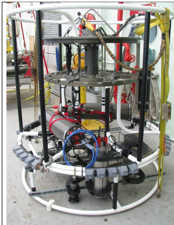
Figure 11. CTD rosette with the Niskin bottles removed and the optical communication hardware installed. The CTD instrument remained installed. The optical communications instrumentation used the SDSL communication protocol to allow for real-time comms with the optical system.
