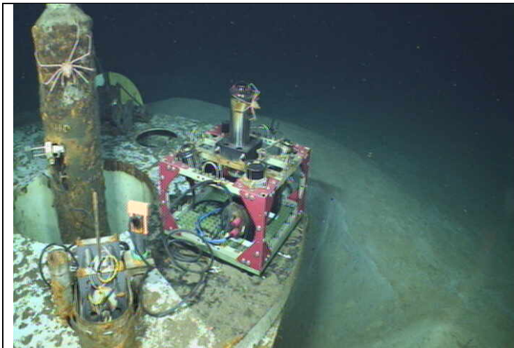
Figure 16. Photo of CORK 857D with optical communication sled plugged into the CORK electronics
