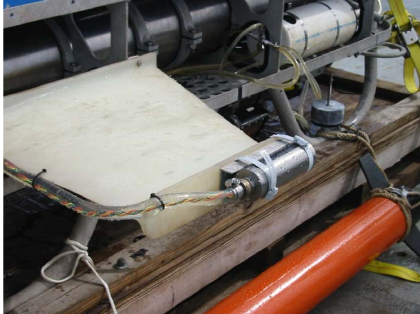
Figure 6. Photograph showing the HMR2300 vector magnetometer mounted to the starboard wing of the sidescan vehicle.
