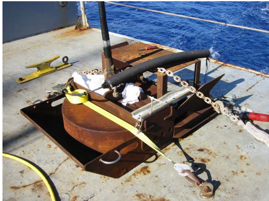
Figure 5. Photograph of the clump weight showing the improvised junction of the fiber-optic cable and neutrally buoyant tow umbilical for DSL-120A.
