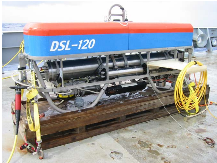
Figure 4. Photograph of the DSL-120A sidescan sonar tow vehicle, port side prior to its first launch. Yellow cable to right is magnetometer tow cable. Fiber-optic umbilical is to the left.
