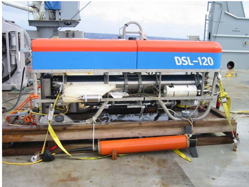
Figure 7. Photograph showing the starboard side of the DSL-120A sidescan vehicle with the KORDI Overhauser magnetometer (orange housing in front slightly disassembled). The HMR2300 vector magnetometer is located on the wing. See Fig. 6.
