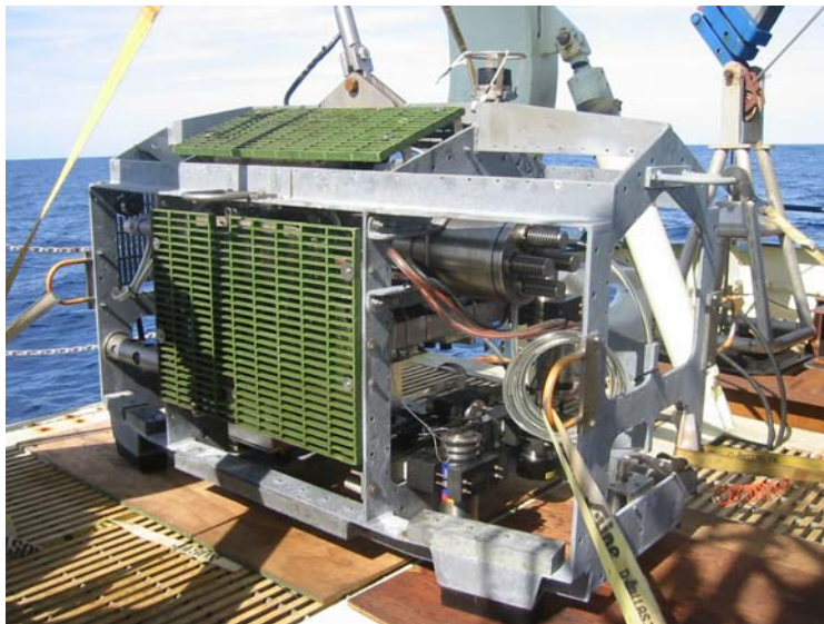
Figure 6. Medea Towed Vehicle is the cable junction box between the main armored cable and the umbilical tether to ROV Jason-2.
