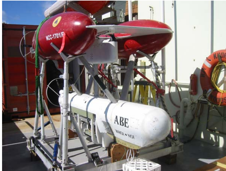
Figure 7. The autonomous underwater vehicle ABE is a self-navigating vehicle that is programmed to follow a prescribed survey mission on the seafloor. ABE navigates by using an acoustic transponder net and a sophisticated seafloor avoidance algorithm. The primary sensor packages used in this study were the Simrad 2000 multibeam sonar (SM2000), magnetometer, digital still camera and a newly added sub-bottom chirp sonar. Note that for this cruise ABE had a depth limit of 3000 meters due to the depth rating of the SM2000 sonar.
