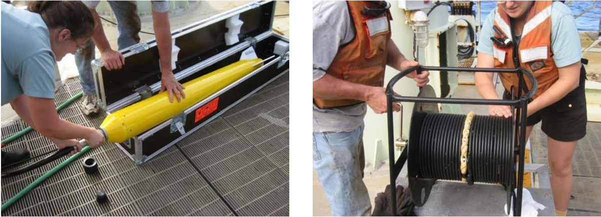
Figure 9. Left shows towed magnetometer sensor. Right photo shows the cable spool.
