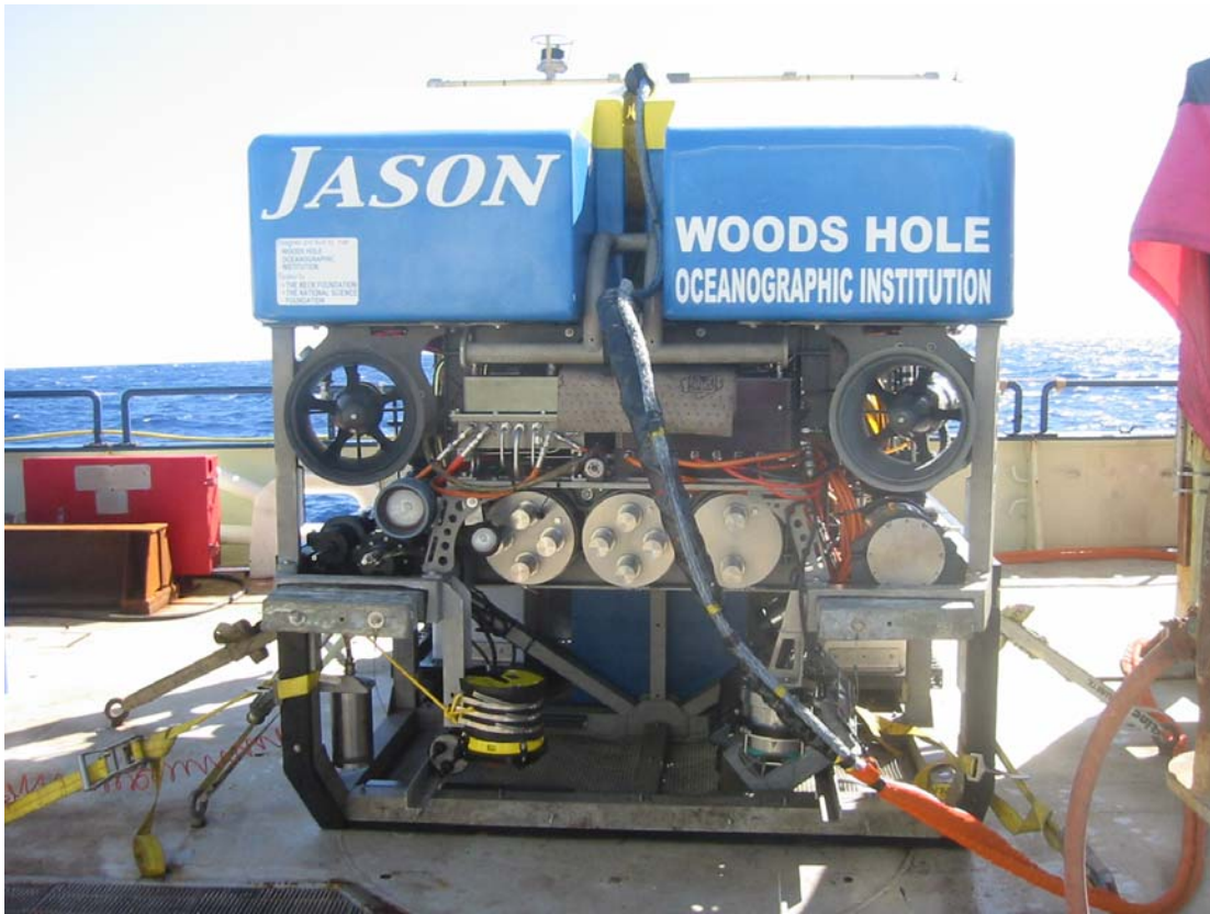
Figure 5. Aft view of Jason-2 showing the aft thrusters and doppler navigation systems. The 1200 khz Doppler had limited range and was supplanted by the 300 Khz Doppler system borrowed from Hanu Singh.
