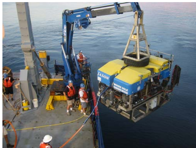
Figure 6b. ROV Jason being launched.
