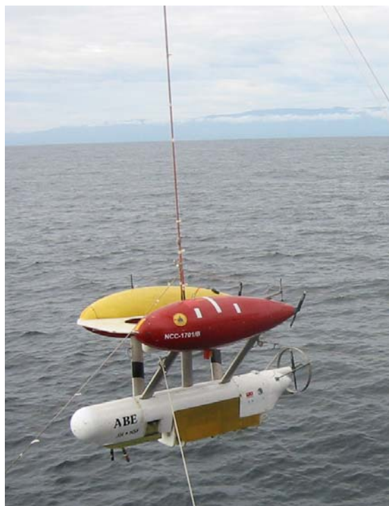
Figure 7. The autonomous underwater vehicle, ABE being recovered after a mission. ABE is a hovering type of vehicle which allows it to survey in rugged terrain.
