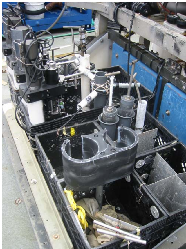
Figure 6a. ROV Jason basket showing 4 gastight water samplers and holders for two major water samplers, along with two push cores and scoop bags.
