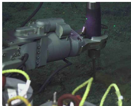
Figure 15. NDSF Heat Flow Probe inserted into sediment.
