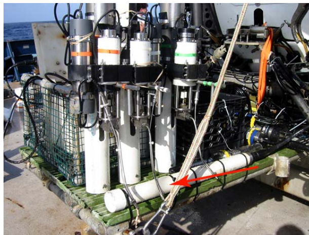
Figure 13. Photograph of Alvin 's basket as configured for this cruise showing placement of the magnetometer (red arrow pointing to long white tube laying on the basket), and Seewald gas-tight water samplers (vertical cylinders with colored tape).
