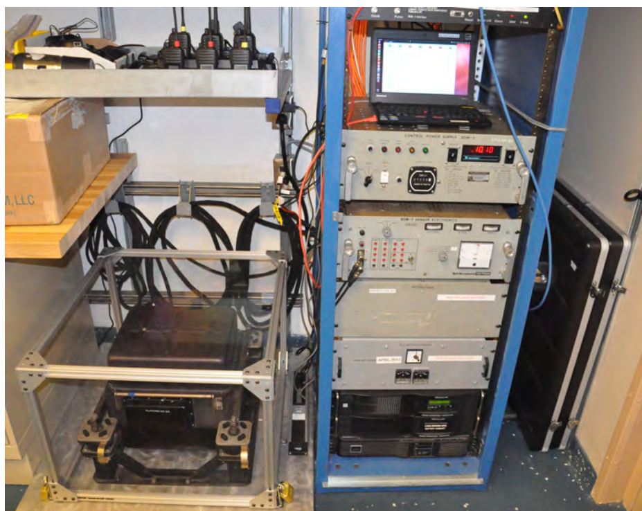
Figure 12. BGM-3 Marine Gravimeter on board the R/V Sikuliaq.
