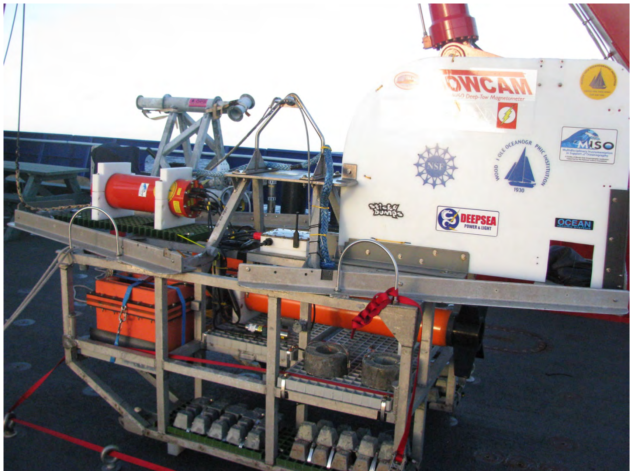
Figure 17. The Deep Tow Magnetometer (DTM) on board the R/V Sikuliaq
