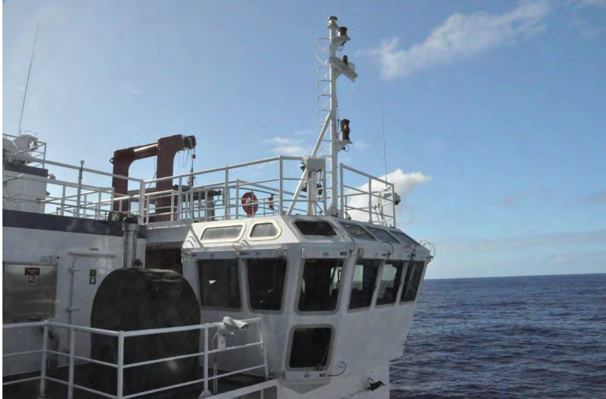
The winch control room overlooks the working deck
