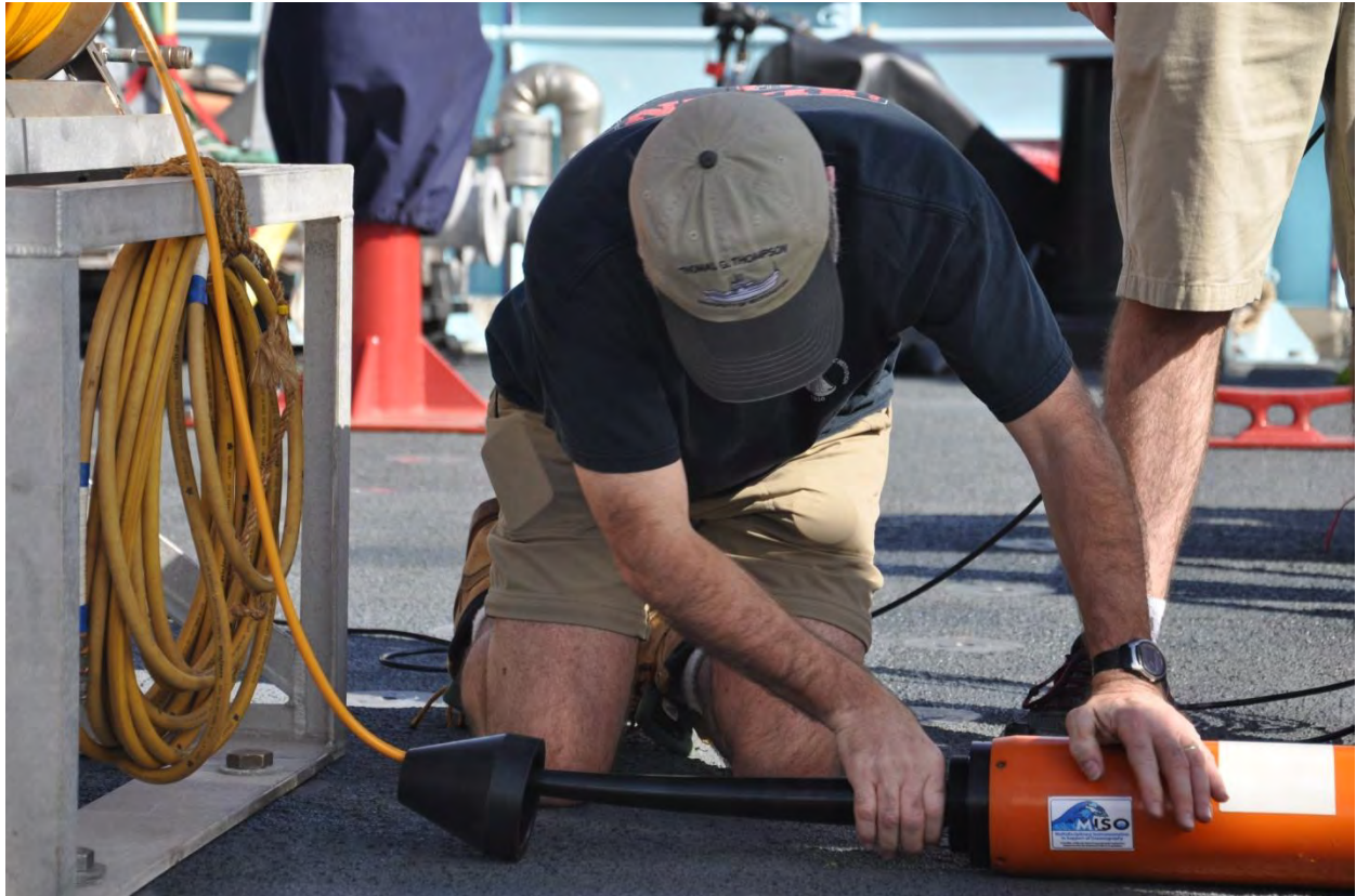
Maurice connects the surface maggie to its tow and data cable
