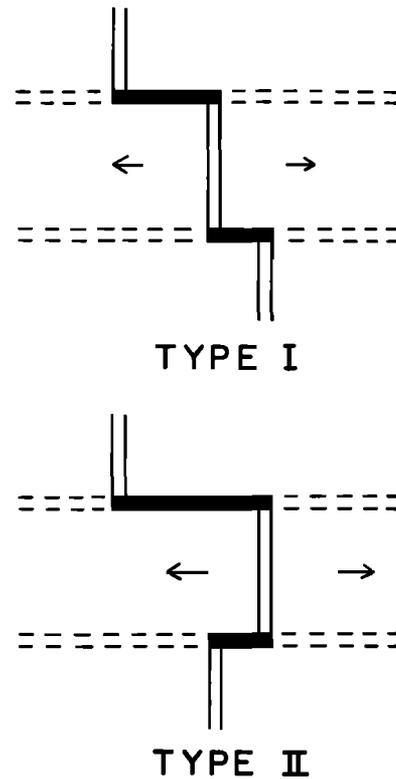
Fig. 7. Two types of ridge-transform segments; the double line represents the ridge segment, the solid line represents the transform fault, and the double dashed line represents the fracture zone.
