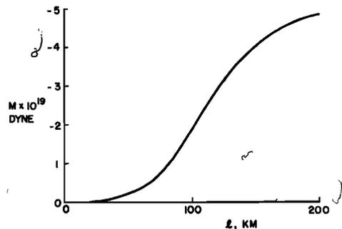
Fig. 5. Bending moment at the center of the ridge segment as a function of the length of the ridge segment.
