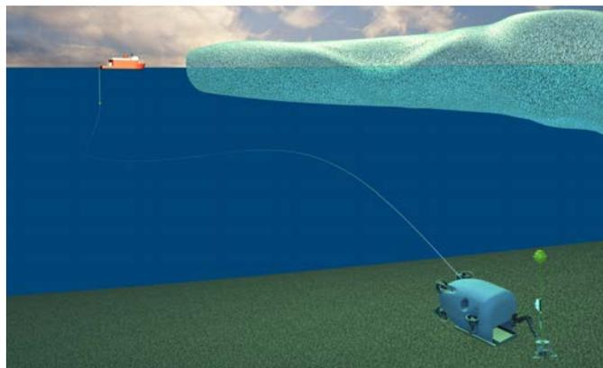
Fig. 1. A schematic representation of operators using *Nereid-UI* to interact with emplaced instrumentation beneath glacial ice kilometers away from the support vessel.
