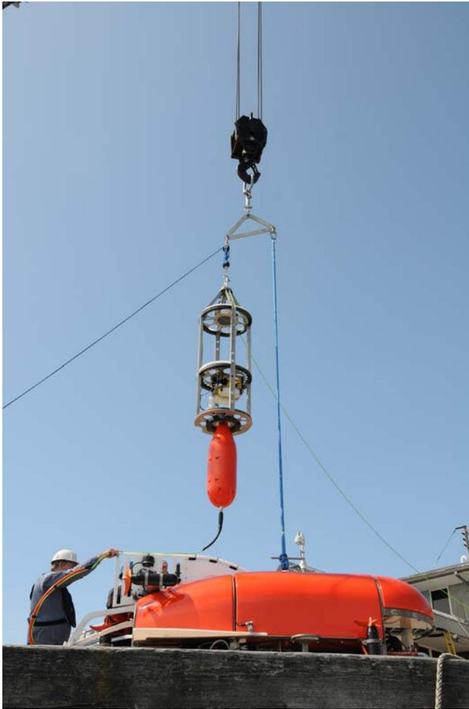
Fig. 3. *Nereid UI* with mated tow-body/depressor ready for launch. The depressor pictured is a prototype borrowed from the *Nereus* project capable of deploying an experimental larger-diameter fiber. We used block-and-tackle rig pictured for dock-trials but will use an air-tugger for trials off *R/V Polarstern* to permit lowering the depressor beyond keel depth.
