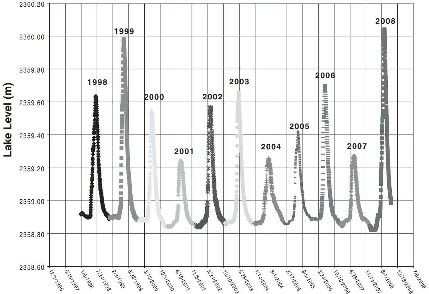
Figure 42. Yellowstone Lake level data and discharge data for the U.S. Geological Survey Fishing Bridge gauging station, downloaded from the National Water Information System (NWIS, [http://nwis.waterdata.usgs.gov/wy/nwis/discharge/?site\\_no=06186500](http://nwis.waterdata.usgs.gov/wy/nwis/discharge/?site_no=06186500)), were fit to a power series regression, enabling calculation of lake level data from the daily discharge data available for the period from 1998 to 2004.
