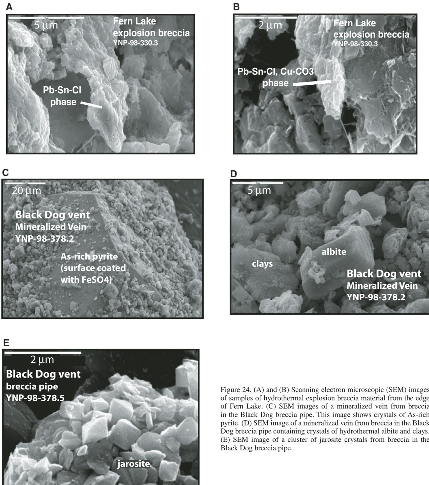
Figure 24. (A) and (B) Scanning electron microscopic (SEM) images of samples of hydrothermal explosion breccia material from the edge of Fern Lake. (C) SEM images of a mineralized vein from breccia in the Black Dog breccia pipe. This image shows crystals of As-rich pyrite. (D) SEM image of a mineralized vein from breccia in the Black Dog breccia pipe containing crystals of hydrothermal albite and clays. (E) SEM image of a cluster of jarosite crystals from breccia in the Black Dog breccia pipe.
