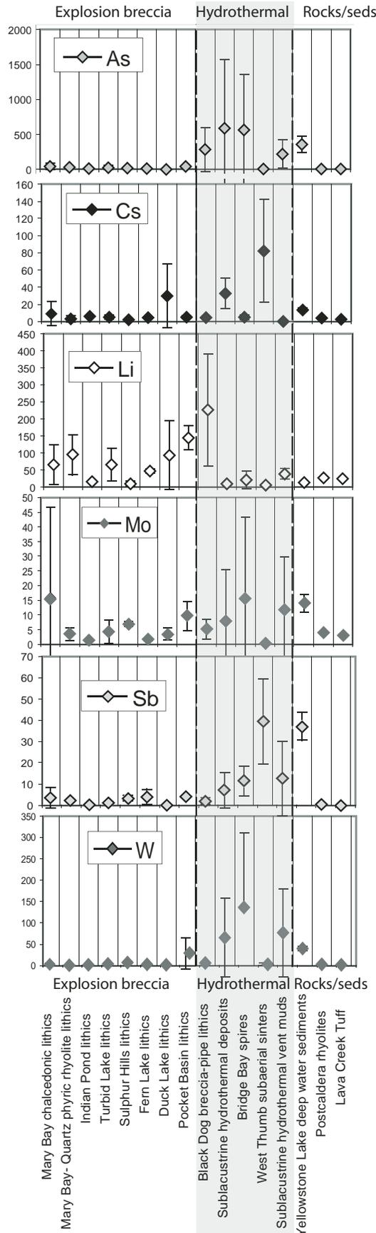
Figure 32. Trace-element distribution for selected geothermal indicator elements in hydrothermal explosion breccia, hydrothermal mineralization, and unaltered rhyolites and lake sediments. These patterns show that the breccias are hydrothermally altered and strongly enriched in As, Li, Mo, Sb, and sometimes Cs and W, like sublacustrine hydrothermal mineralization.
