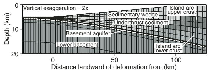
**Figure 2.** Portion of grid used in finite element model; model extends from 150 km seaward to 250 km landward of deformation front. The 600-m-thick aquifer at top of the subducting crust facilitates up dip heat transport. The thermal effect of high Nusselt number ( $Nu$ ) circulation in the aquifer is simulated using high thermal conductivity.
