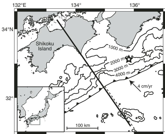
**Figure 1.** Locations of deformation front in Nankai Trough (barbed line) and cross section modeled (bold line), which is along the axis of a fossil spreading center (dashed line). Thin lines are bathymetry in meters. Arrow indicates convergence between Philippine Sea plate and southwest Japan. Star marks epicenter of 1946 Nankaido earthquake. Inset shows study area offshore southern Japan.
