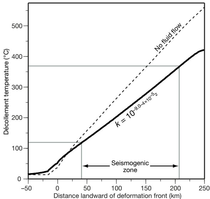
**Figure 4.** Modeled temperatures along the megathrust. With preferred aquifer permeability (thick solid line), seismogenic zone defined by Sagiya and Thatcher (1999) extends from  $\sim 125$  to  $\sim 365^\circ \text{C}$ .
