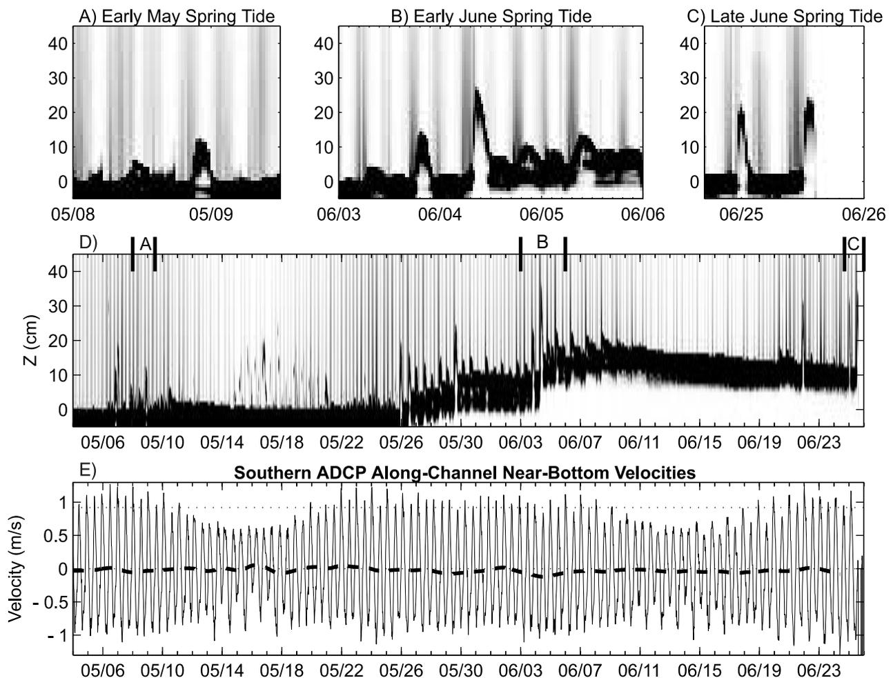
**Figure 8.** (a–c) Three periods of ABS data showing transient fluid mud deposits as delineated by regions labeled A, B, and C in Figure 8d. (e) ADCP data from 2.5 mab with low-pass-filtered data (dashed line).
