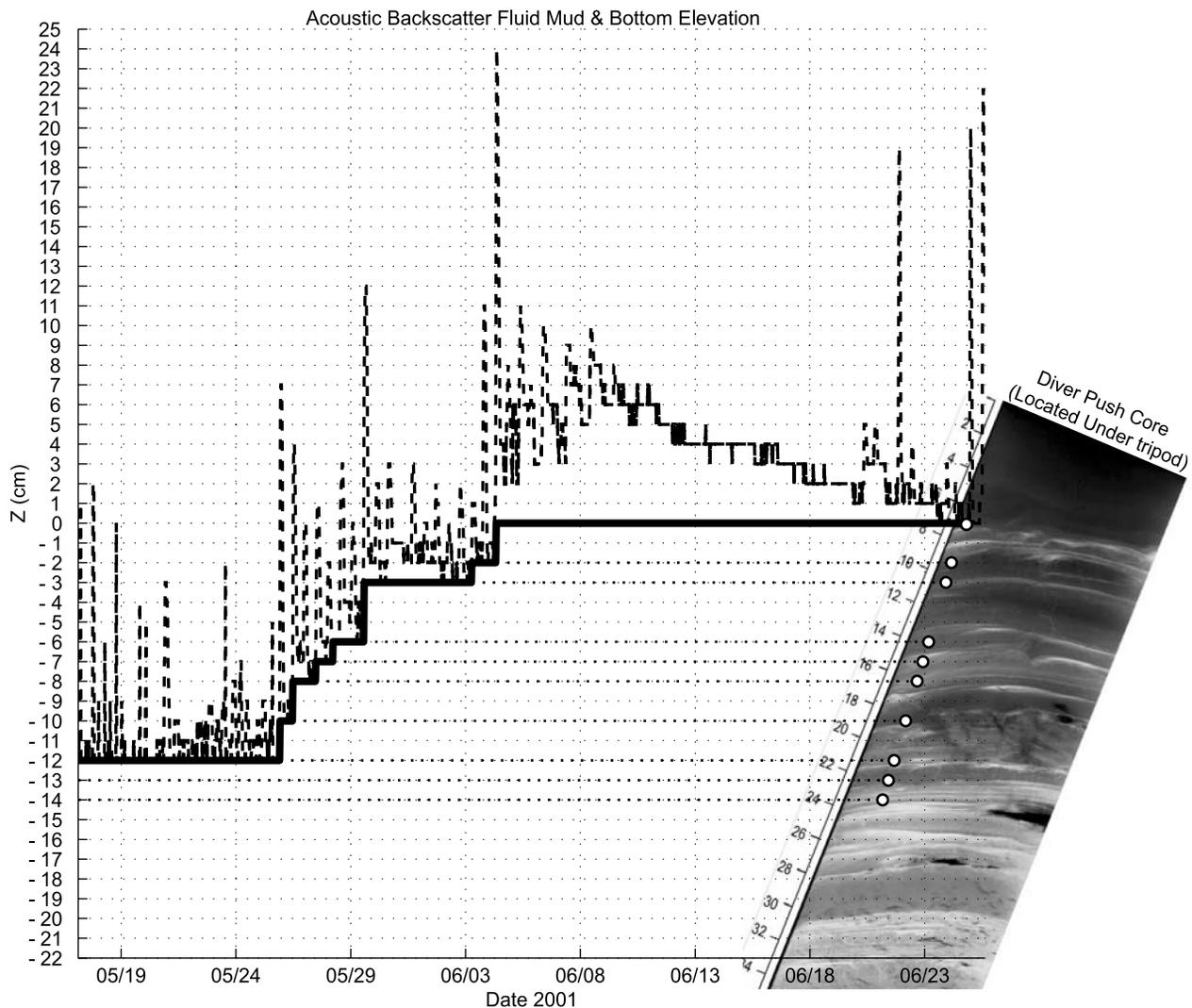
**Figure 18.** (left) Elevation of the bed (thin solid line) and the fluid mud transient deposit (dashed line) from ABS data. The thick black line (with dotted lines to align surfaces to the core) represents consecutive erosional surfaces that could potentially be seen in a core as fine sand to coarse silt laminae. (right) An X-radiograph negative from a core taken directly under the tripod during recovery aligned with the ABS elevation data.
