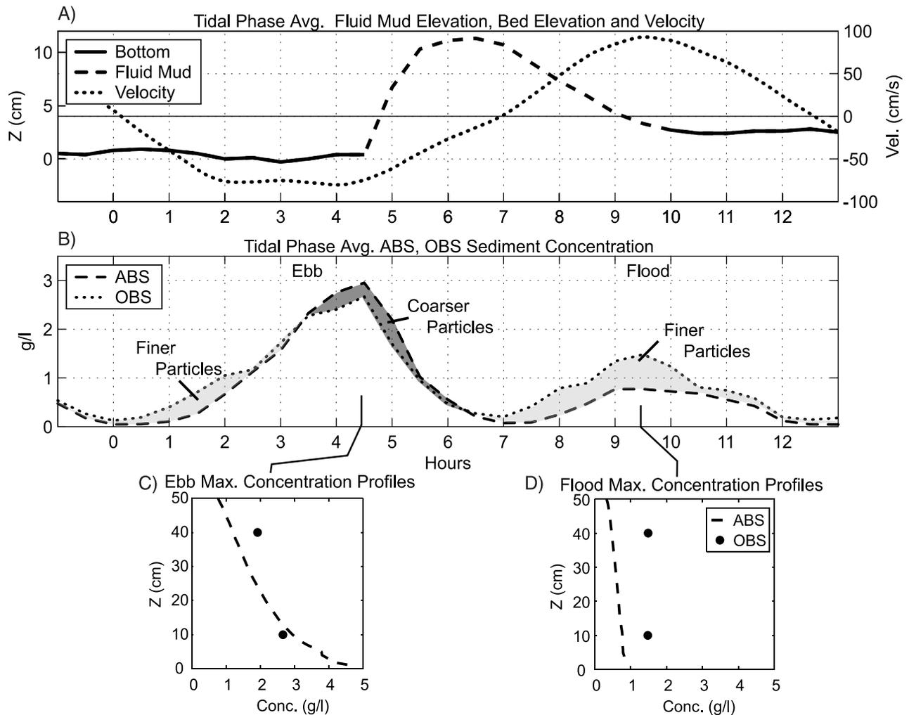
**Figure 17.** (a) Phase-averaged bed elevation, fluid mud, and velocity for tidal cycles with  $>1$  cm of mud accumulation during the period of high deposition from 26 May to 5 June. (b) Phase-averaged ABS and OBS suspended sediment concentration estimates from 20 cmab for the same tidal cycles as in Figure 17a. (c, d) Vertical profiles of suspended sediment concentration estimates from the ABS (dashed line) and OBS (dots) at maximum concentration during ebb and flood.
