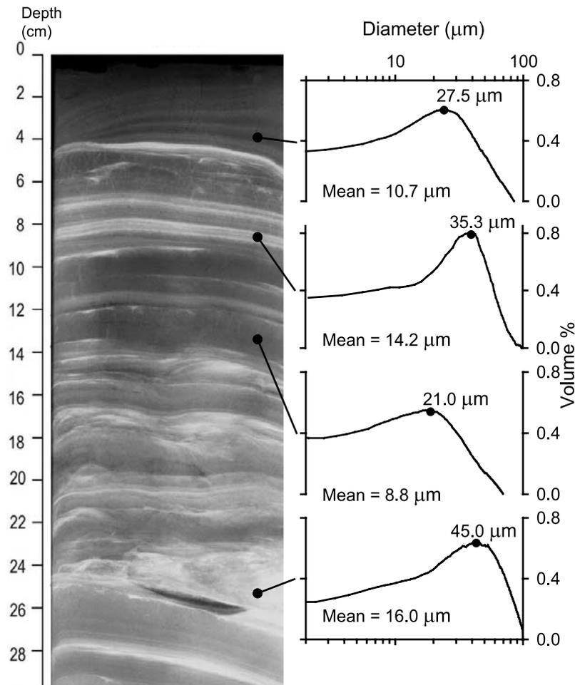
**Figure 12.** (left) An X-radiograph negative from a core taken by divers adjacent to the southern tripod at the end of the deployment on 25 June. Light areas are higher-density sand and silt layers, and dark areas are mud. (right) Grain size distributions for coarser and finer grain size laminae within the bed. Mean and mode grain sizes are shown for each distribution.
