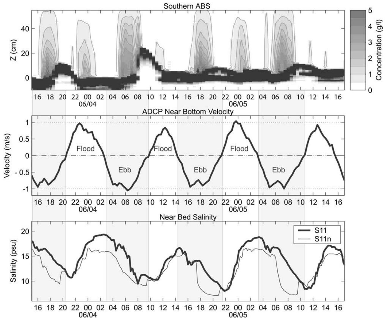
**Figure 9.** (top) Four tidal cycles of ABS data showing transient deposits of fluid mud. Contours of sediment concentration are spaced  $0.5 \text{ g L}^{-1}$  apart. (middle) Acoustic Doppler current profiler (ADCP) tidal velocity from 2.5 mab. (bottom) Salinity from the southern depositional site tripod (S11) and the small tripod located 500 m to the north (S11n).
