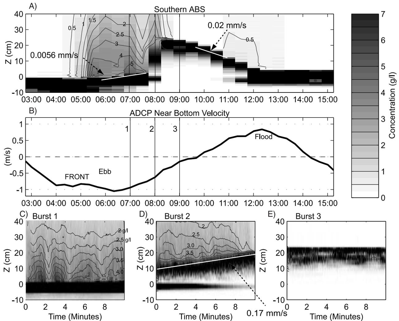
**Figure 10.** (a) Burst-averaged half hourly sampled ABS data from 4 June. Contours of sediment concentration are spaced  $0.5 \text{ g L}^{-1}$  apart. (b) ADCP tidal velocity 2.5 mab. (c–e) Three bursts of 1 Hz sampled ABS data at times 1, 2, and 3, as indicated in Figures 10a and 10b. Figure 10c shows a turbulent suspension. Figure 10d shows the rising mud-water interface as sediment deposits, and Figure 10e shows some internal acoustic structure in the recent deposit.
