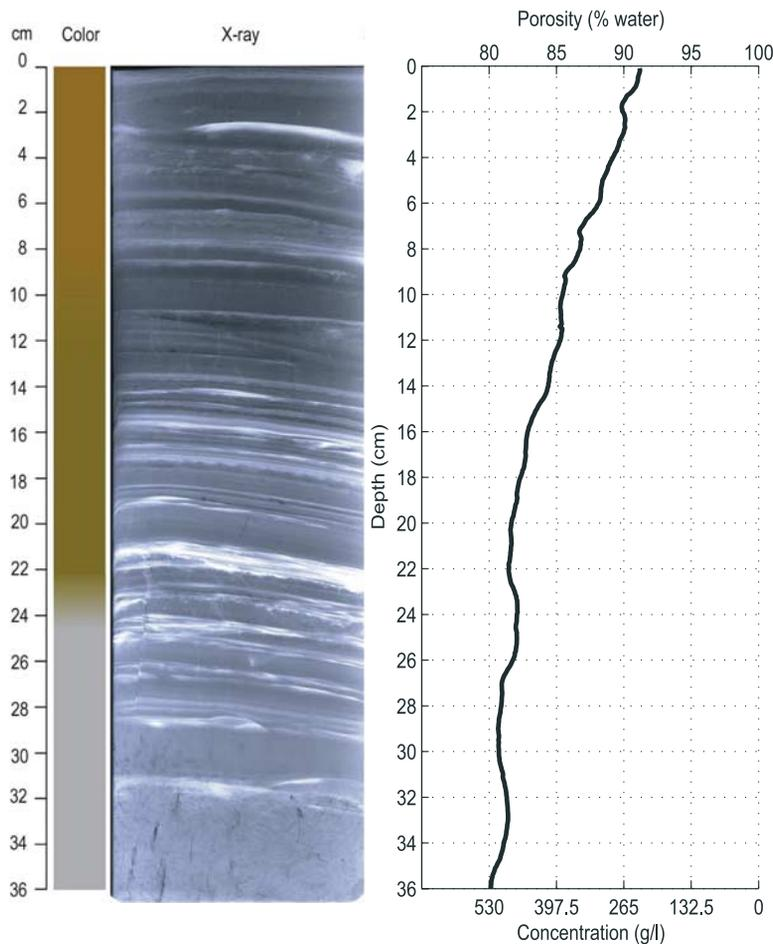
**Figure 6.** (left) An X-radiograph negative and photo color from a box core taken  $\sim 30$  m from the southern tripod 2 days after the end of the deployment in June. Light areas in the X-radiograph are higher-density very fine sand and silt layers, and dark areas are clay and silt. (right) Porosity profile from resistivity measurements from the same box core.
