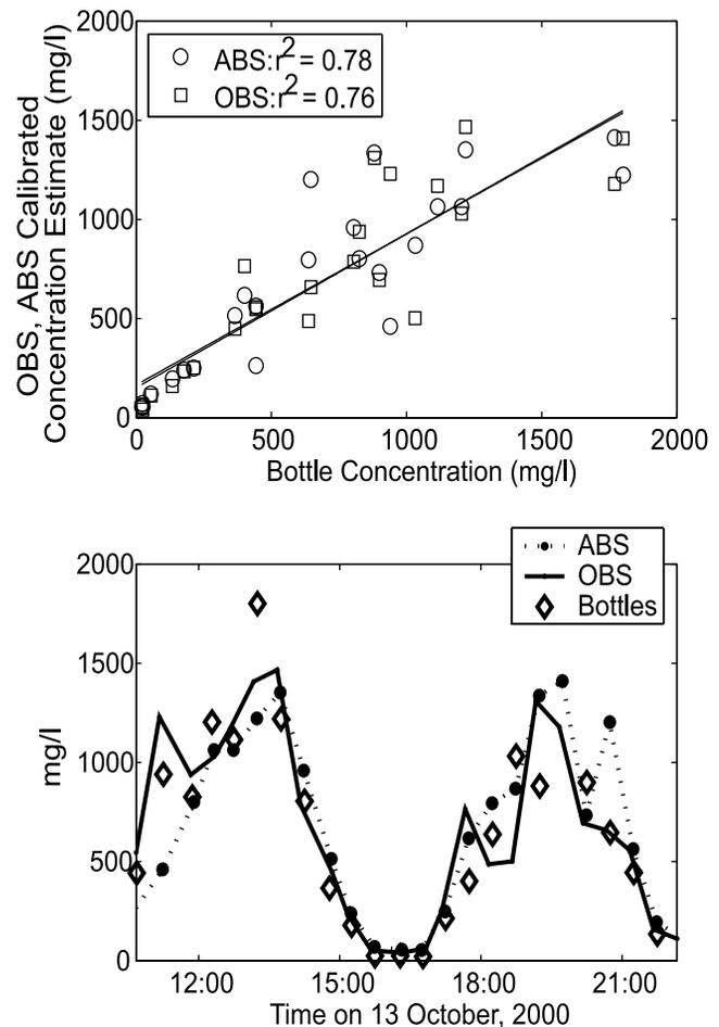
**Figure 2.** (top) Calibrated optical backscattering sensor (OBS) and acoustic backscattering sensor (ABS) concentration estimates from the southern depositional site tripod versus bottle samples taken near the tripod at 0.5 meters above bottom (mab). (bottom) ABS and OBS concentration estimates and bottle concentration time series.
